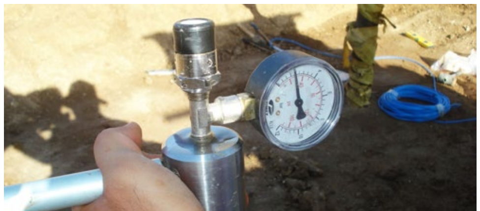
Saturation of HAE filter with saturation device
